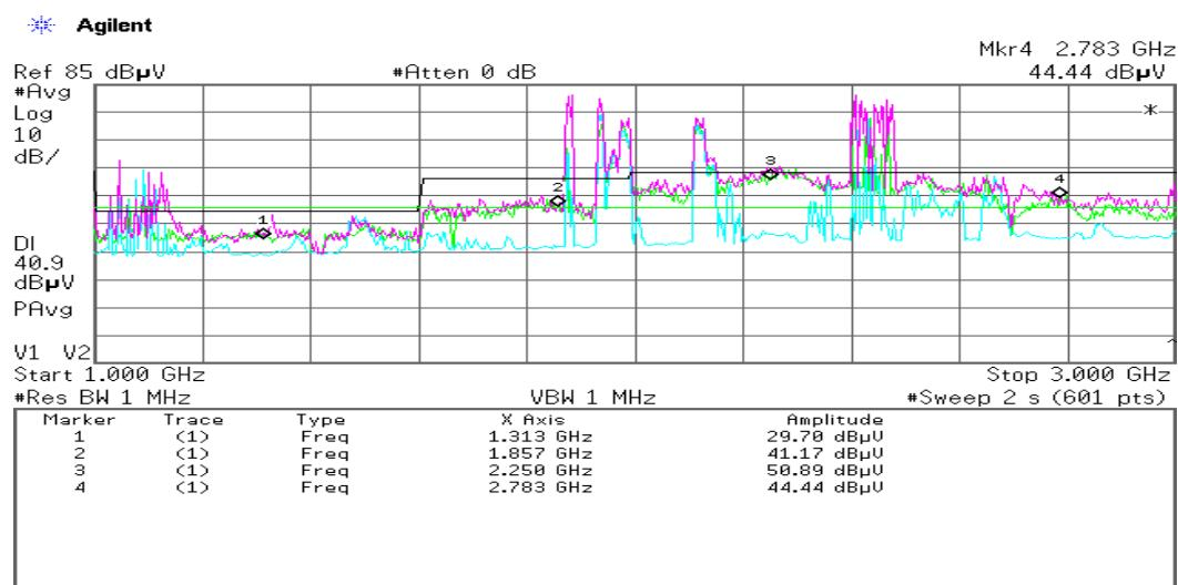
Since the OATS measurement was conducted with manual position changes ( interval 45 degree). Only the worst points were collected from ambient noise. Not practical to provide all OFB spurious emission plots. This plot is for illustration purpose.
