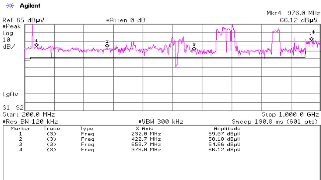
Since the OATS measurement was conducted with manual position changes ( interval 45 degree). Only the worst points were collected from ambient noise. Not practical to provide all OFB spurious emission plots. This plot is for illustration purpose. The difference between QP and Peak Readings is about 13~18dB.
