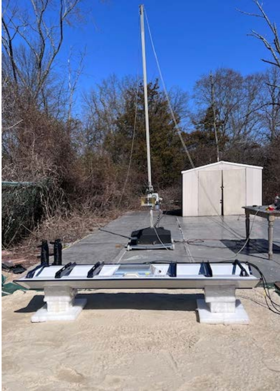
Above 1GHz ( when needed, 1m measurement for low emission signals)
