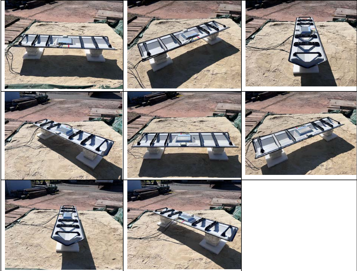
EUT Positions with 45 Degree Interval
