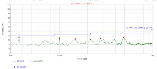
Suspected List Freq. Factor Limit Margin Height Reading Level Angle NO. Polarity [MHz] [dB] [dBµV/m] [dBµV/m]  $[dB\mu V/m]$ [dB] [cm] [°] 36.796797 -14.57 51.19 36.62 40.00 3.38 100 293 Vertical 99.90991 -14.70 49.64 34.94 43.50 8.56 100 293 Vertical 148.45845 50.99 43.50 100 280 -18.14 32.85 10.65 3 Vertical 4 214.48448 -14.76 45.56 30.80 43.50 12.70 100 138 Vertical 5 -12.69 46.07 46.00 100 276.62662 33.38 12.62 314 Vertical 488.29829 -7.91 43.58 35.67 46.00 100 6 10.33 179 Vertical
