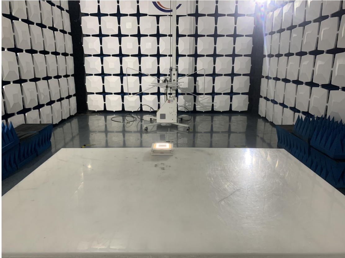
Above 1GHz for radiated emission test setup
