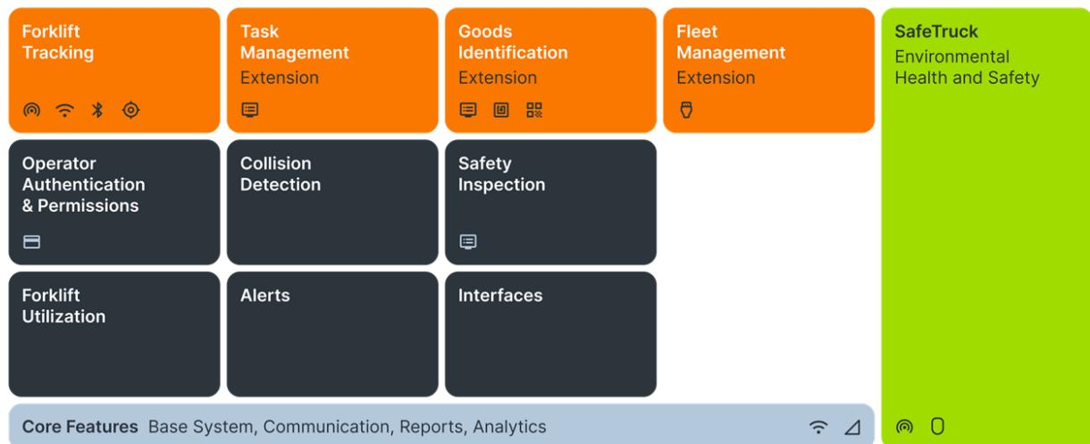
The combination of the SafeTruck and the SmarTruck systems enables an integrated and vendor-independent solution that provides utilization tracking, operator authorization, and safety control functionalities for forklifts and other vehicles involved in material-handling processes. Due to the flexible and modular design, various functional configurations can be supported.
