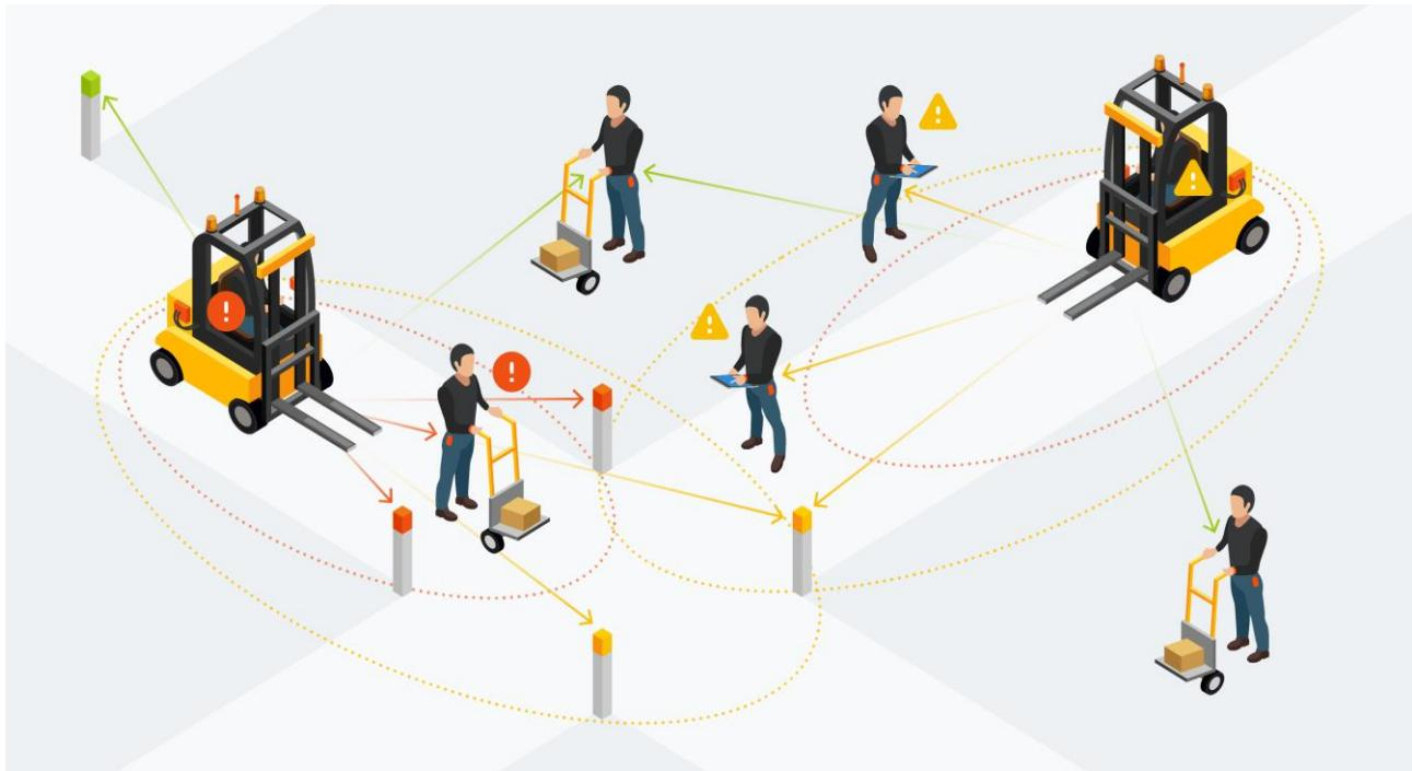
To enable the distance-based proximity detection of pedestrians on forklifts and other vehicles, the workers are provided with handheld SafeTag components. The SafeTag components participate in the distance measurements initiated by the SafeRadar components and automatically activate the built-in audible, visual, and haptic warning signals to alarm individuals about the proximity of forklifts and other vehicles (based on the preconfigured activation zones).
