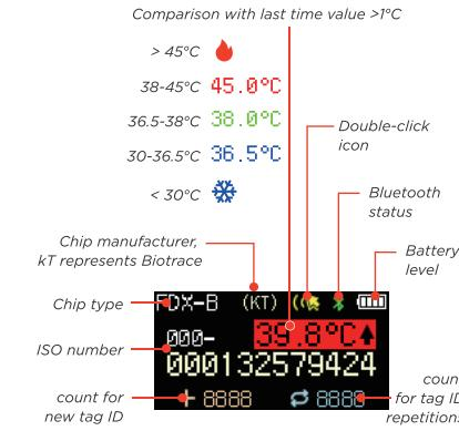
On SCAN menu to press button to start chip reading for 10 seconds. A transponder is detected, the reader emits a 'beep' and displays the chip infor
