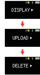
On RECORD menu, press the button to enter the sub-menu, on the sub-menu, double-click to navigate the sub-menu from DISPLAY, UPLOAD to DELETE.
