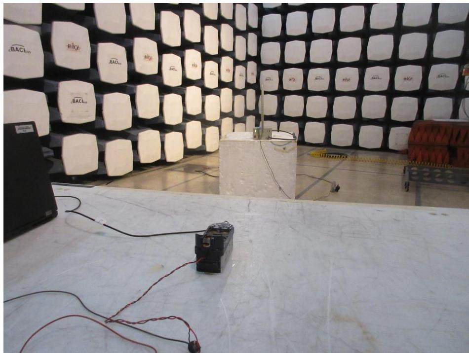
**1.5. EUT Test Setup at 3 Meters Front View (30 MHz – 1 GHz)**
