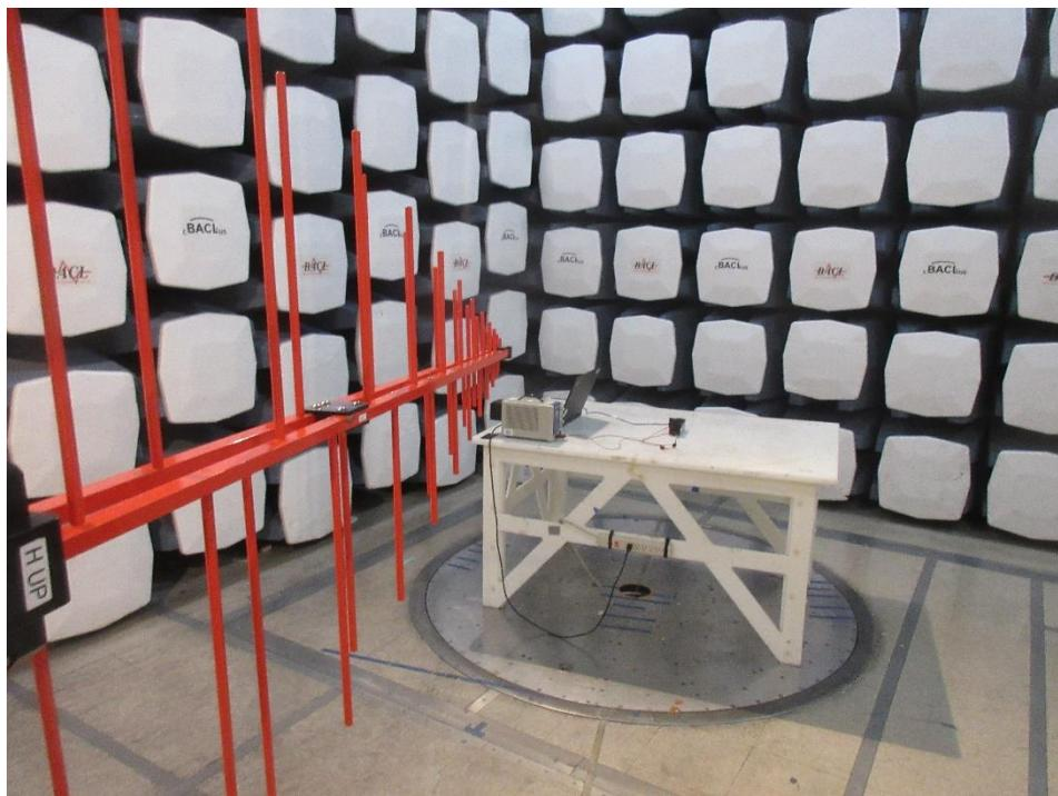
**1.6. EUT Test Setup at 3 Meters Rear View (30 MHz – 1 GHz)**
