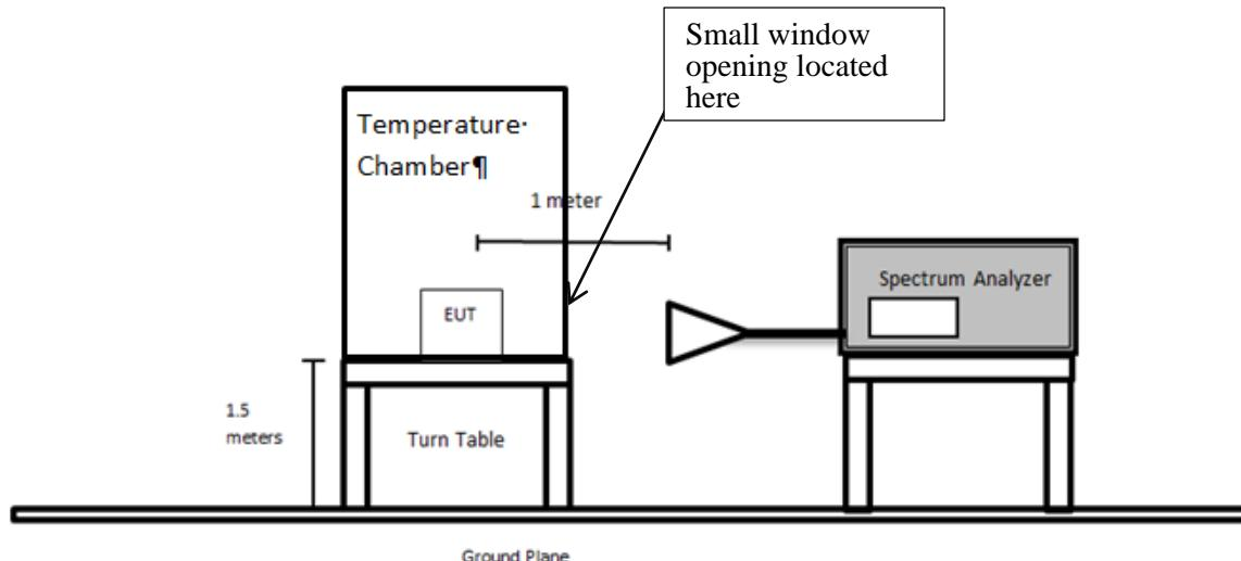
**Note: Small window opening is located on the outside of the chamber which permits receive antenna to make measurements on EUT**
