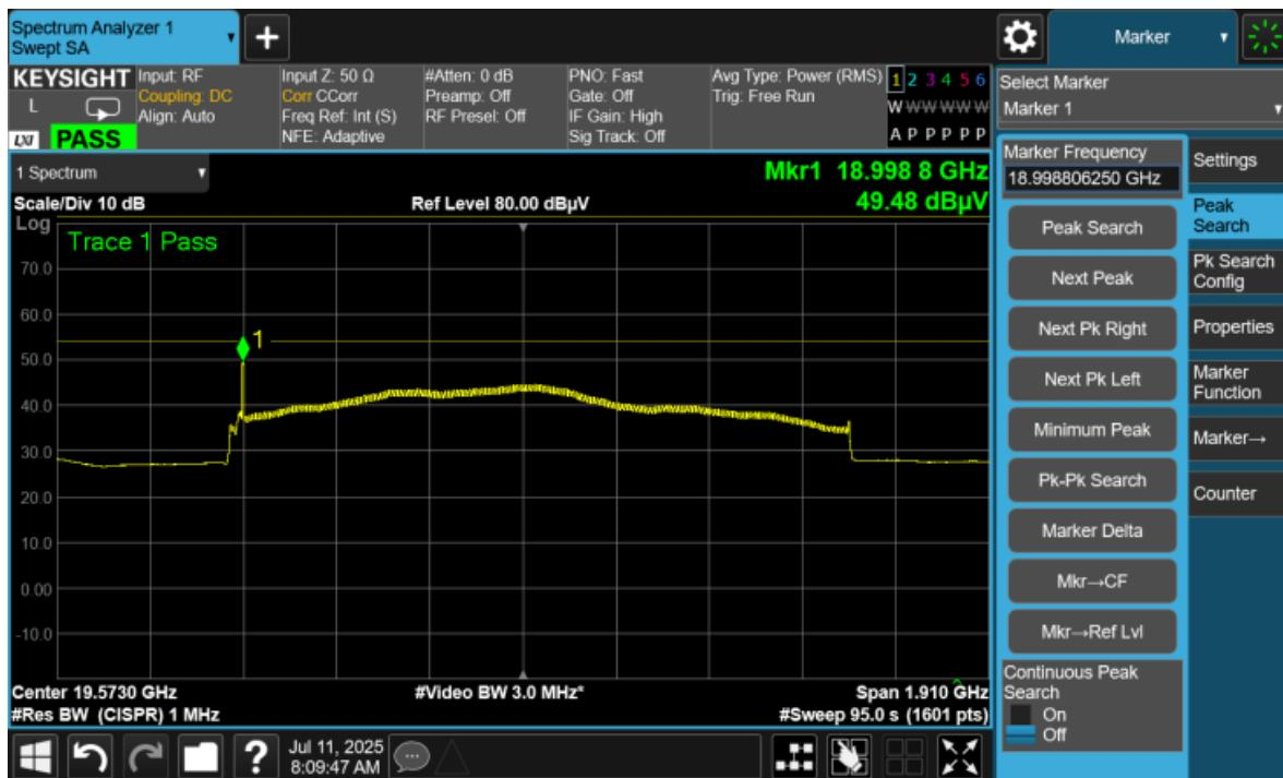
**26.5-40 GHz Worst Case, Measured at 3 meters***Reference Average noise floor plot to show that noise floor is more than 6dB below average limit requirements.*
