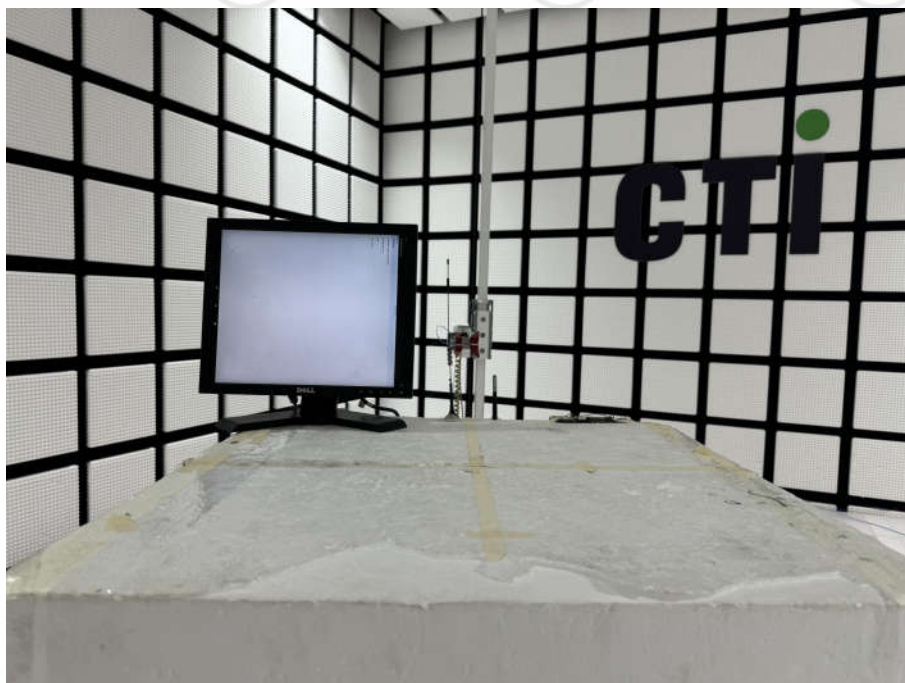
Radiated spurious emission Test Setup-2(Above 1GHz)
