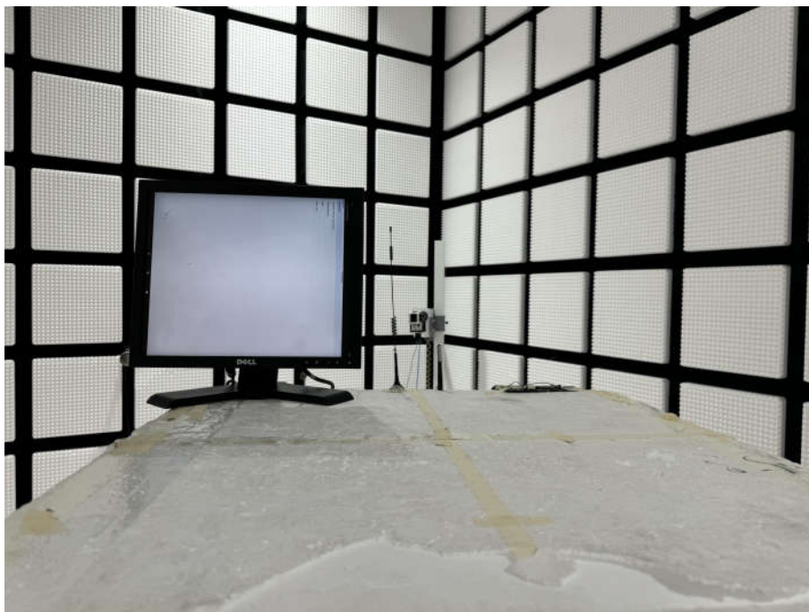
Radiated spurious emission Test Setup-3(Above 18GHz)
