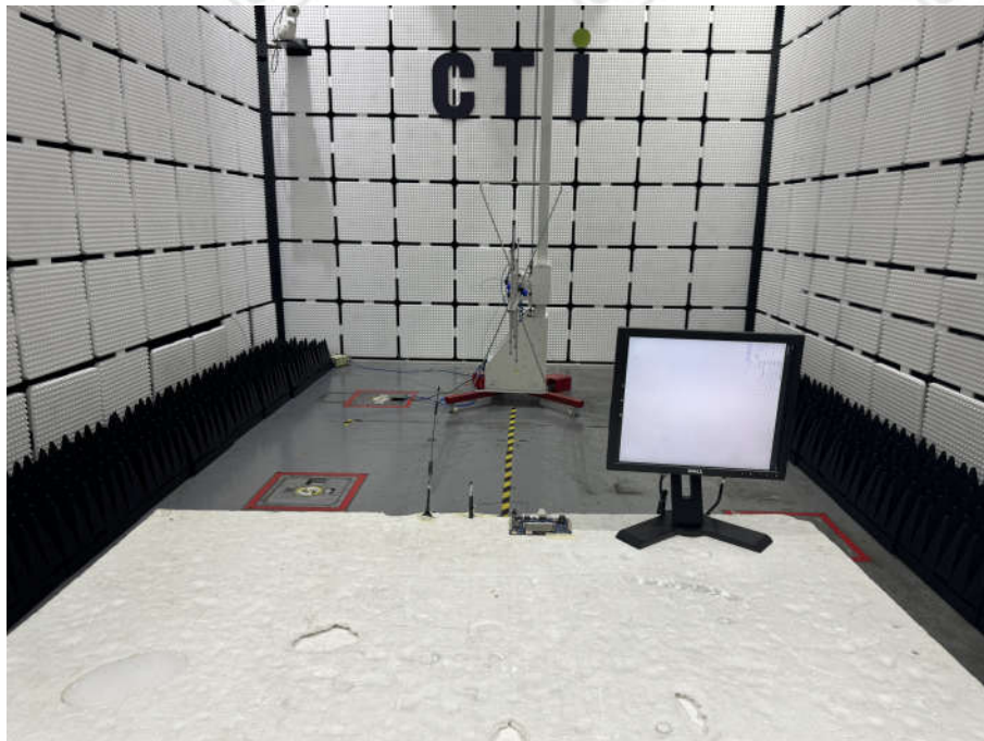
Radiated spurious emission Test Setup-1(Below 1GHz)
