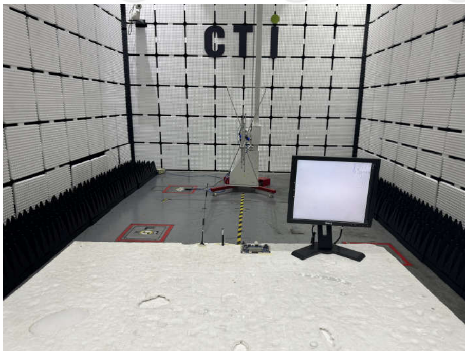
Radiated spurious emission Test Setup-1(Below 1GHz)
