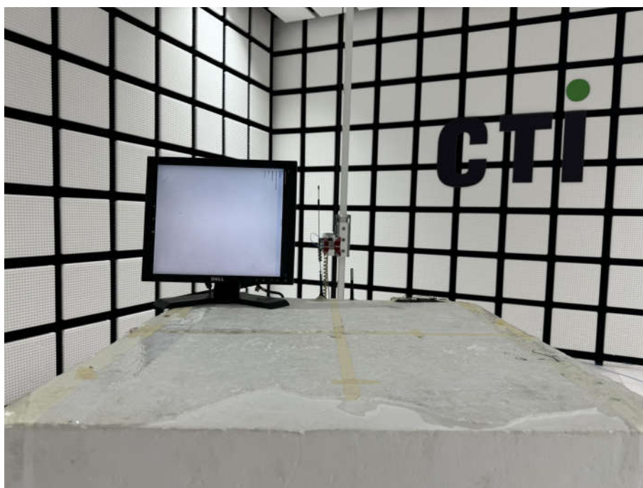
Radiated spurious emission Test Setup-2(Above 1GHz)
