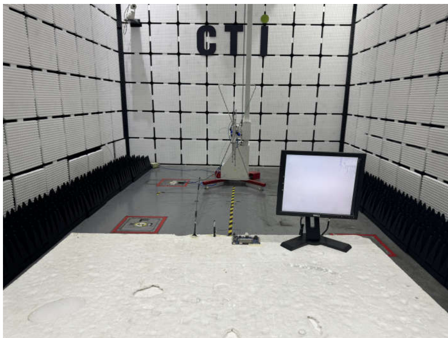
Radiated spurious emission Test Setup-1(Below 1GHz)
