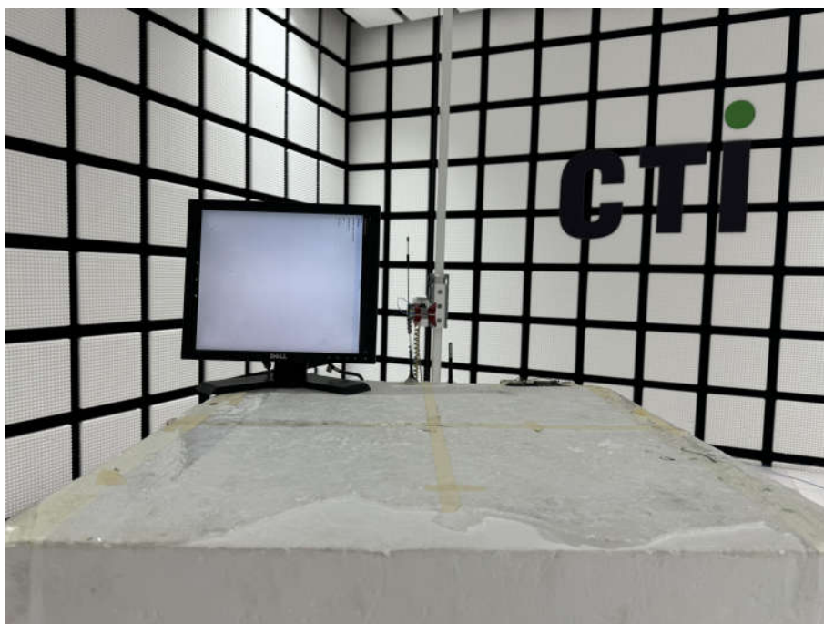
Radiated spurious emission Test Setup-2(Above 1GHz)
