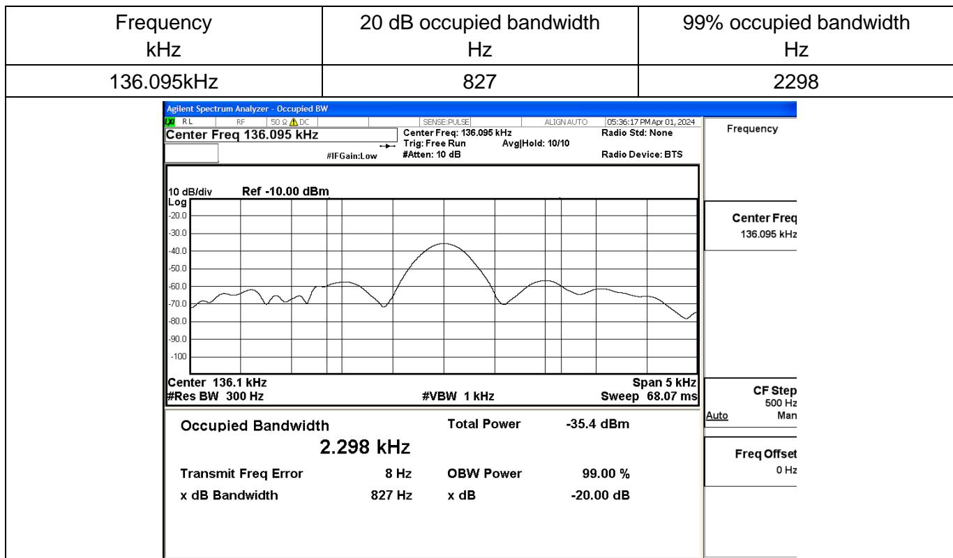
**Note:** Because the measured signal is CW-like, adjusting the RBW per C63.10 would not be practical since measurement bandwidth will always follow the RBW. The RBW is set to 300 Hz to perform the occupied bandwidth test.
