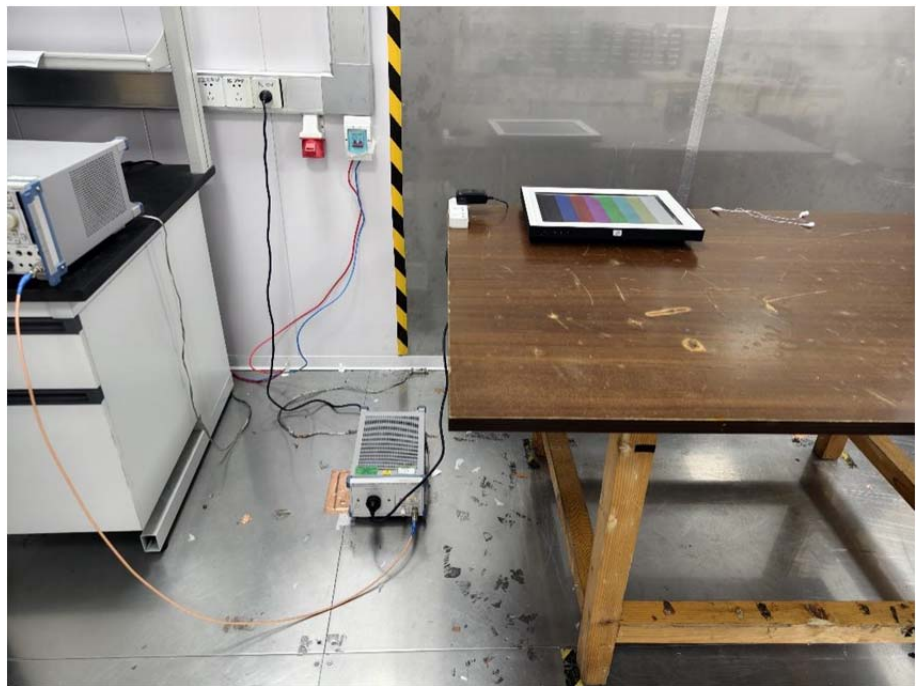
Conducted Emission Test Setup
