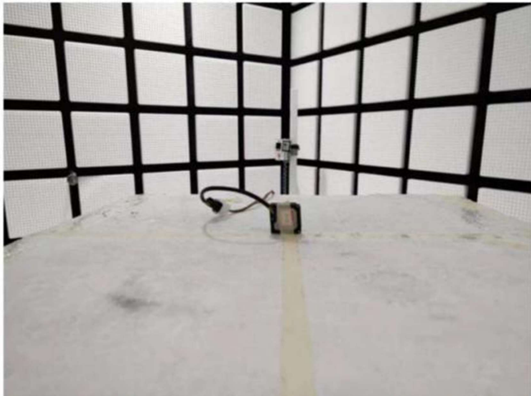
Radiated spurious emission Test Setup-3(18GHz-41GHz)
