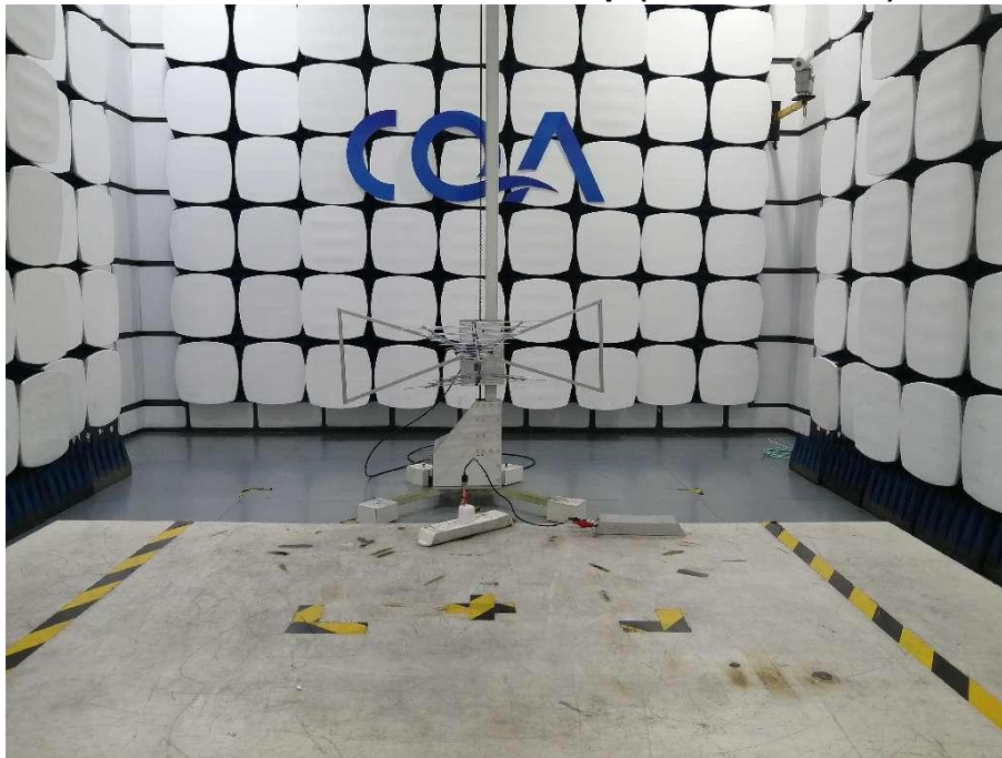
Radiated emission Test Setup (30MHz~1GHz)
