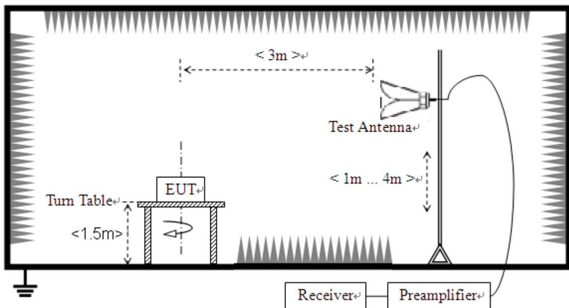
The EUT is placed on a non-conducting table 80 cm above the ground plane for measurement below 1 GHz; 1.5 m above the ground plane for measurement above 1 GHz. The antenna to EUT distance is 3 meters. The EUT is configured in accordance with ANSI C63.10. The EUT is set to transmit in a continuous mode.
