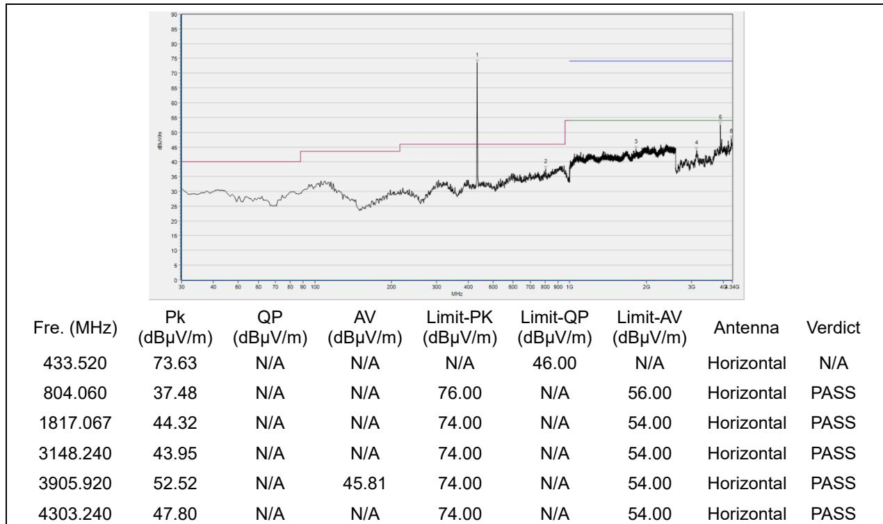
(433.92 MHz, Antenna Horizontal, 30 MHz to 5 GHz)
