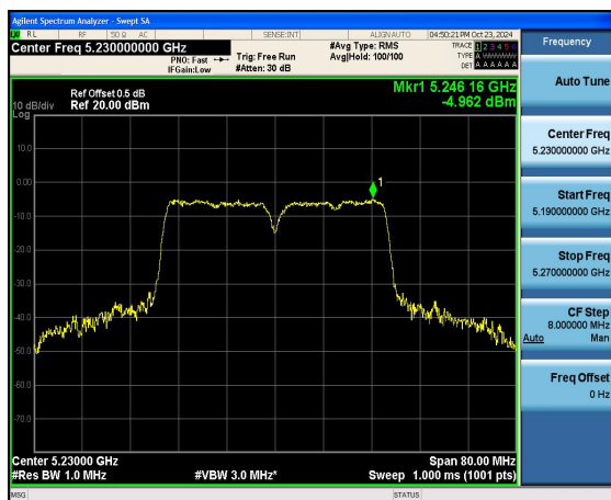
(802.11n40) PSD plot on channel 46
