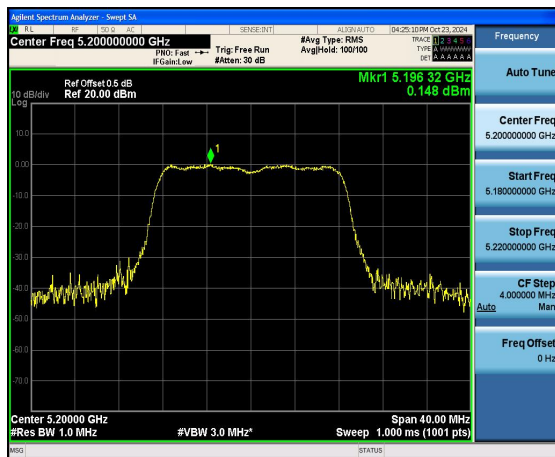
(802.11a) PSD plot on channel 48
