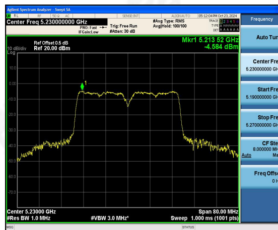
(802.11ac40) PSD plot on channel 46
