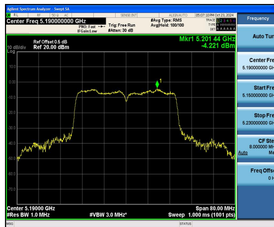
(802.11ac40) PSD plot on channel 38
