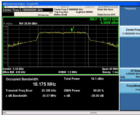
(802.11 n20) 26dB Bandwidth plot on channel 36
