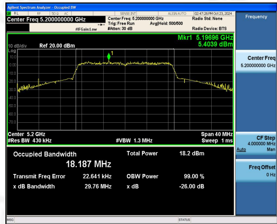
(802.11 n40) 26dB Bandwidth plot on channel 38
