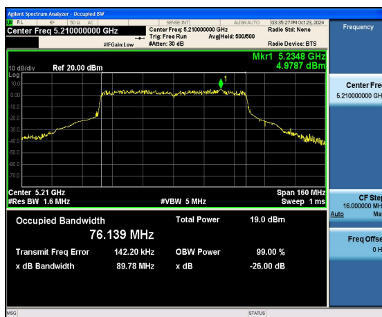
(802.11 ac80) 26dB Bandwidth plot on channel 42
