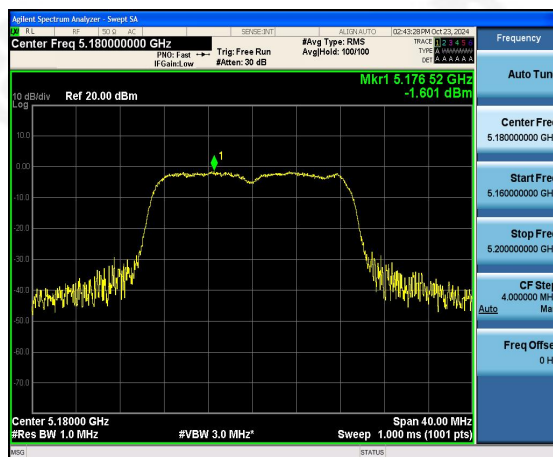
(802.11n20) PSD plot on channel 40
