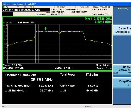
(802.11 ac40) 26dB Bandwidth plot on channel 46
