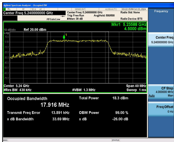
(802.11ac20) 26dB Bandwidth plot on channel 40
