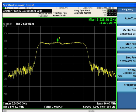
(802.11n20) PSD plot on channel 48
