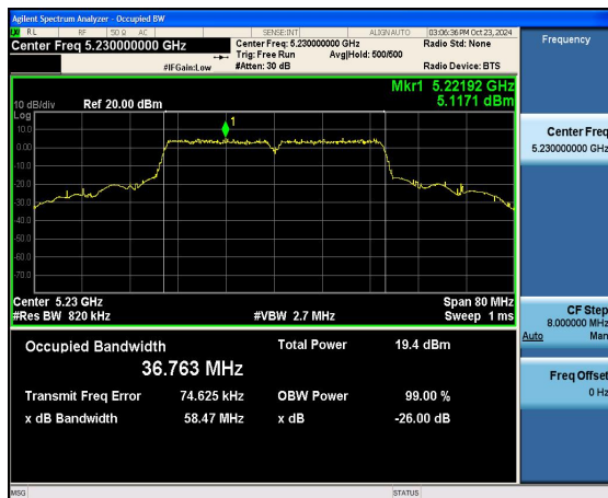
(802.11 n20) 26dB Bandwidth plot on channel 48
