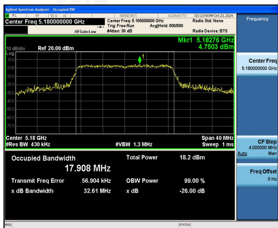
(802.11ac20) 26dB Bandwidth plot on channel 40
