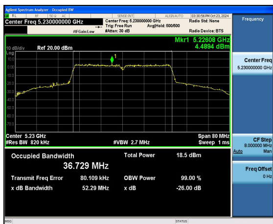
(802.11ac20) 26dB Bandwidth plot on channel 48
