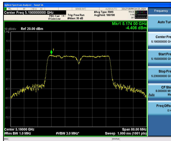
(802.11ac40) PSD plot on channel 46
