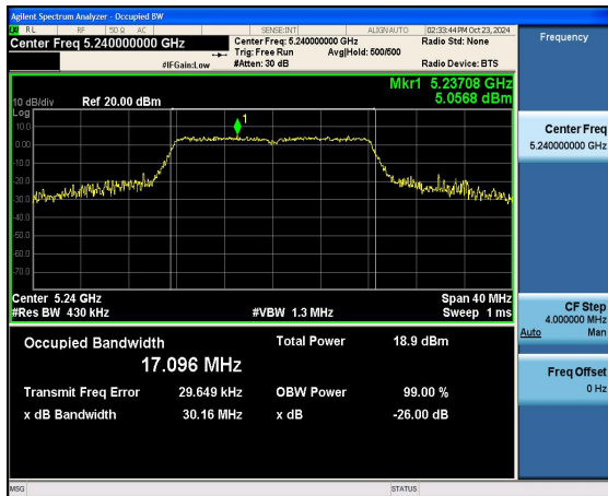
(802.11 a) 26dB Bandwidth plot on channel 48
