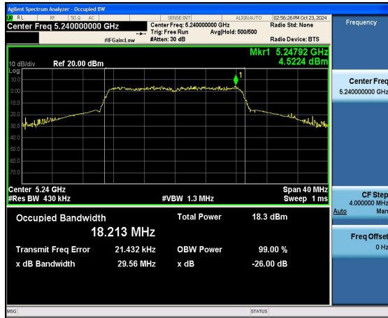
(802.11 n20) 26dB Bandwidth plot on channel 48
