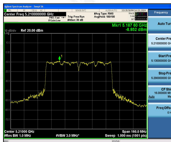
(802.11ac80) PSD plot on channel 42
