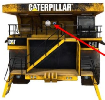
In this instance the RCM is positioned in the middle of the machine on a bracket.
