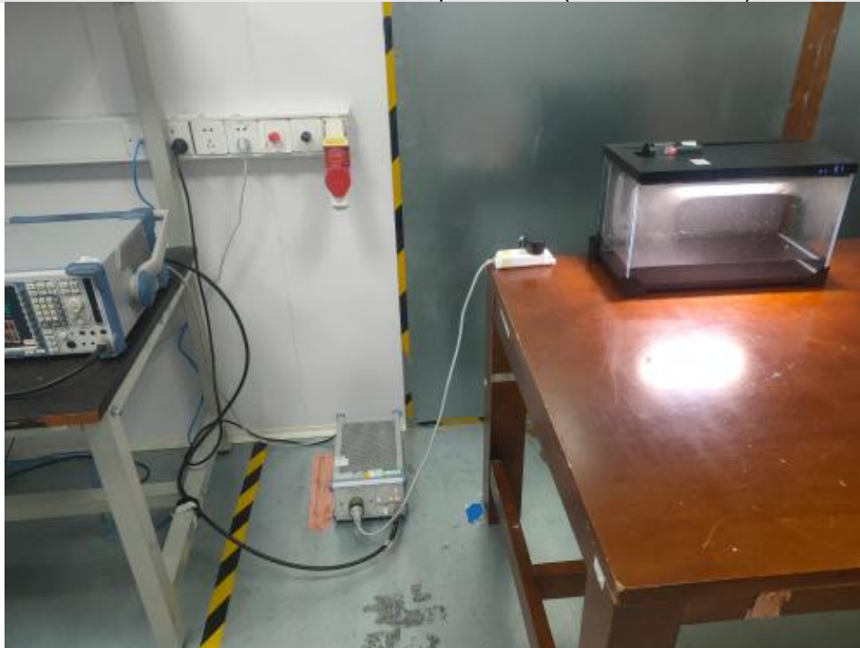
Conducted emissions at AC power line (150kHz-30MHz)
