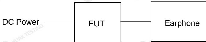
Operation of EUT during above 1GHz Radiation testing:
