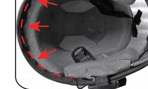
Route the left and right speaker wires inside the helmet lining.
