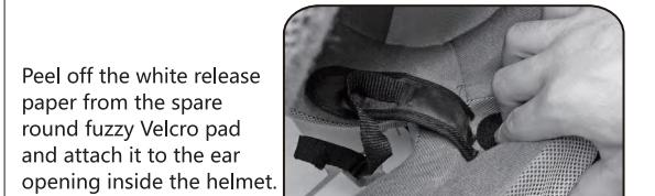
Peel off the white release paper from the spare round fuzzy Velcro pad and attach it to the ear opening inside the helmet.
