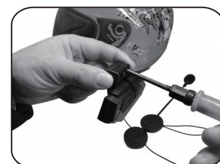
Fig.2 Move the clip and align it on the left side of the helmet Edge in.
