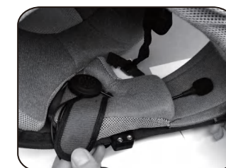
Fig.6 Stick the left horn to the magic The microphone is attached as shown in the picture.
