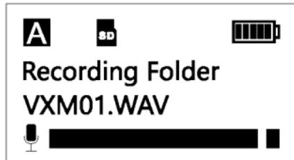
Press SET button to enter recording folder, use the "+" and "-" to choose needed recording file, then press SET button to playback recording file via headphone monitor, press again to exit
