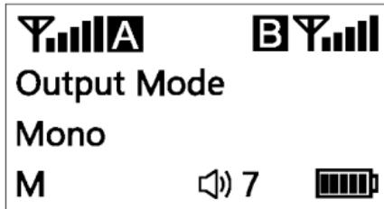
The output mode can be set to mono or stereo, the default is mono
