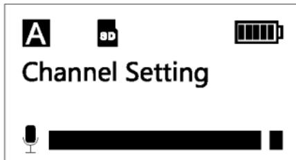
Press the SET button to enter the menu, use the "+" and "-" to select the channel you need then press the SET button to confirm, the default is CH01
