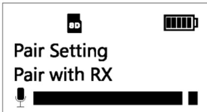
Set to pair with the receiver, the screen will display "Pairing", after successful pairing, it will back to pairing setting screen
