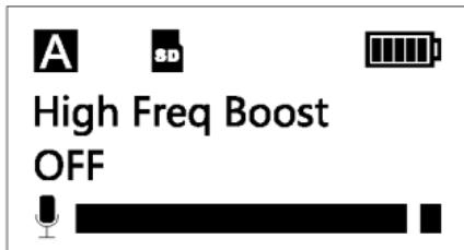
High Frequency Boost with 5 level: **OFF**; **+1dB**; **+2dB**; **+3dB**; **+4dB**, the default is OFF
