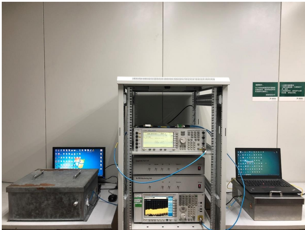
DFS Set-up Photo: Slave and Spectrum Analyzer
