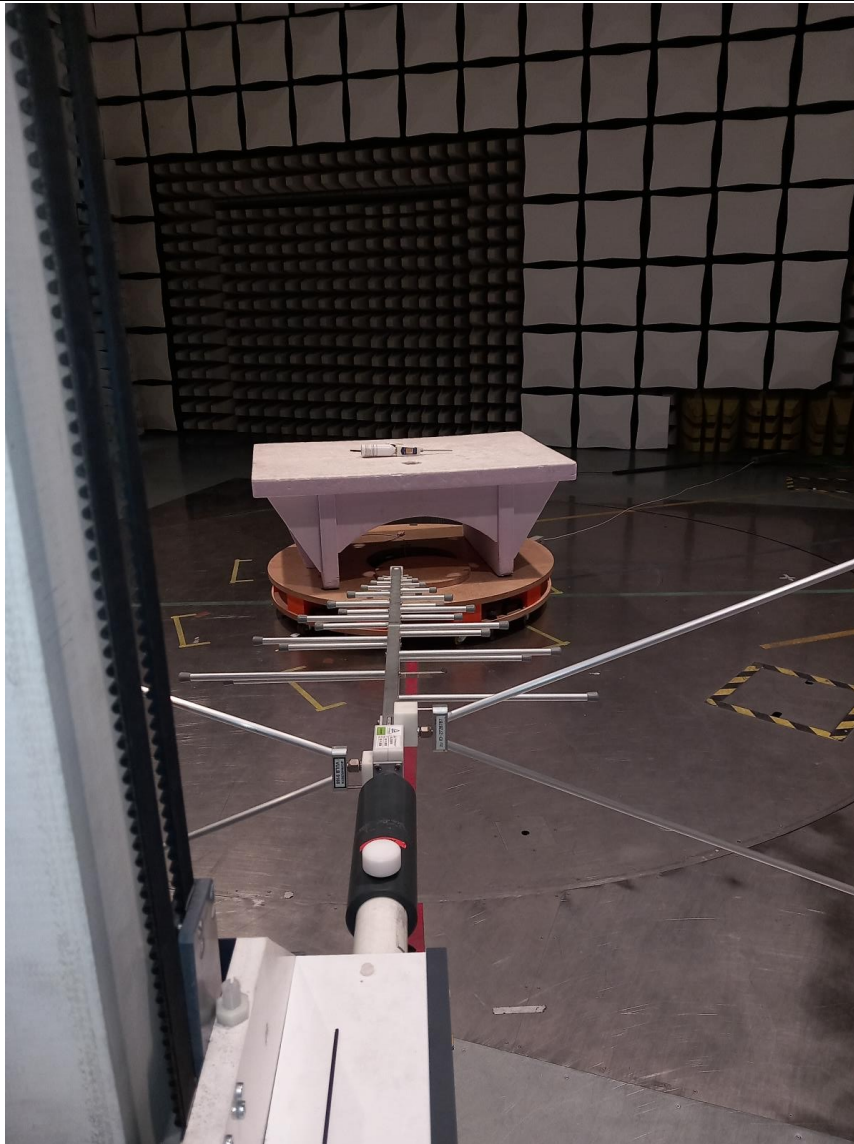
Test Setup: Radiated Measurements (30MHz - 1GHz) Horizontal polarization
