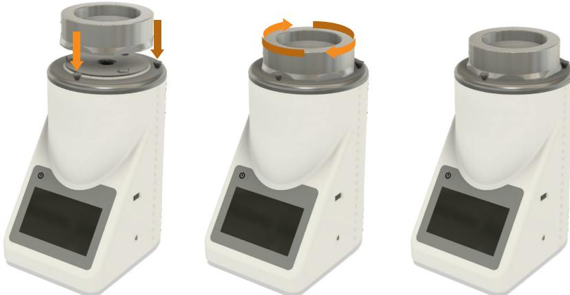
To fit the sieve head, align the flat spots at the bottom of the sieve head with the bayonet pins on the top of the iVAS Roam, then lower the sieve head onto the iVAS Roam and twist until the sieve head is held securely. To remove the sieve head, twist until it becomes loose and lift off.
