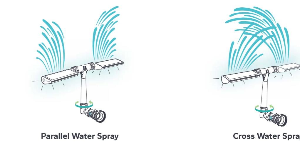
After rotating the riser and adjusting the spray angle, repeat steps 7-8 to swap the left and right fountains, ensuring the solar panel faces upward.
