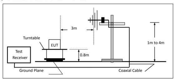
(c) For radiated emissions above 1000MHz
