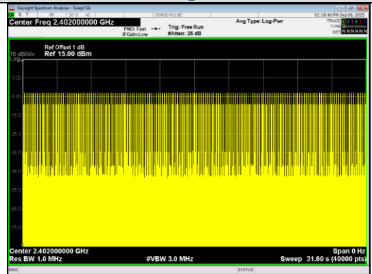
Number of Pulses in 31.6 seconds \pi/4 DQPSK_2-DH1
