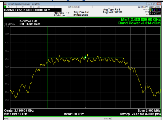
Average Output Power \pi/4 DQPSK_Channel 78
