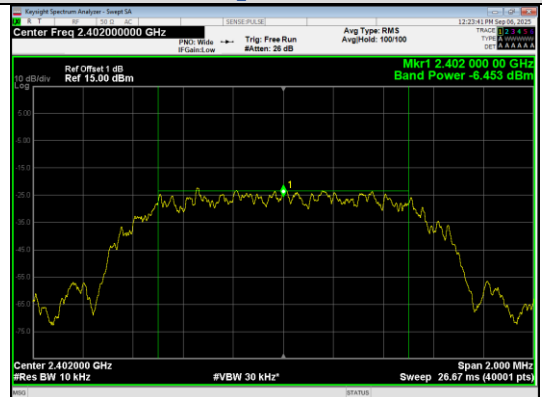
Average Output Power \pi/4 DQPSK_Channel 0
