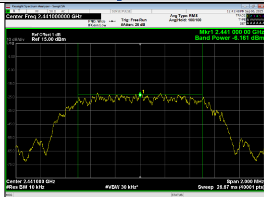
Average Output Power \pi/4 DQPSK_Channel 39
