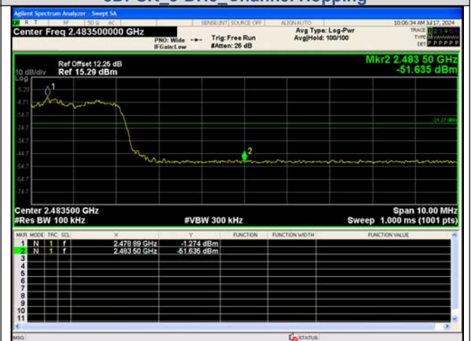
Out Of Band Emission(Right) 8DPSK_3-DH5_Channel Hopping
