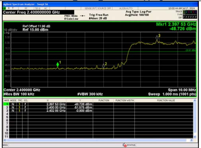
Out Of Band Emission(Left) \pi/4 DQPSK_2-DH5_Channel Hopping
