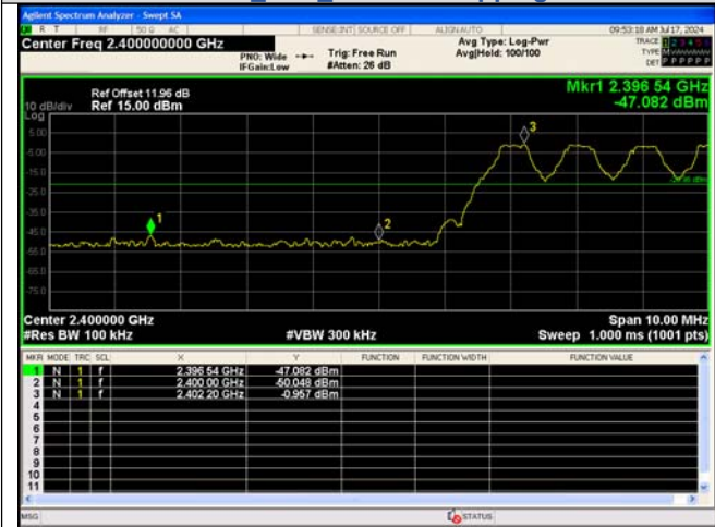
Out Of Band Emission(Left) GFSK_DH5_Channel Hopping
