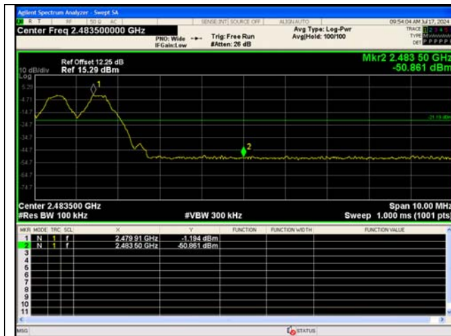
Out Of Band Emission(Right) GFSK_DH5_Channel Hopping
