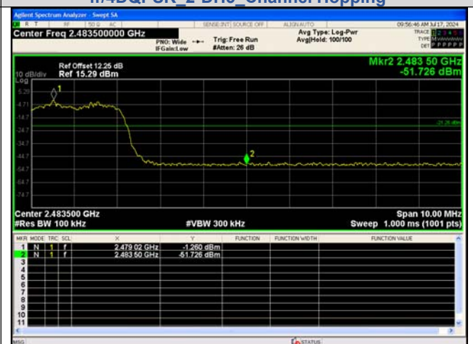
Out Of Band Emission(Right) \pi/4 DQPSK_2-DH5_Channel Hopping
