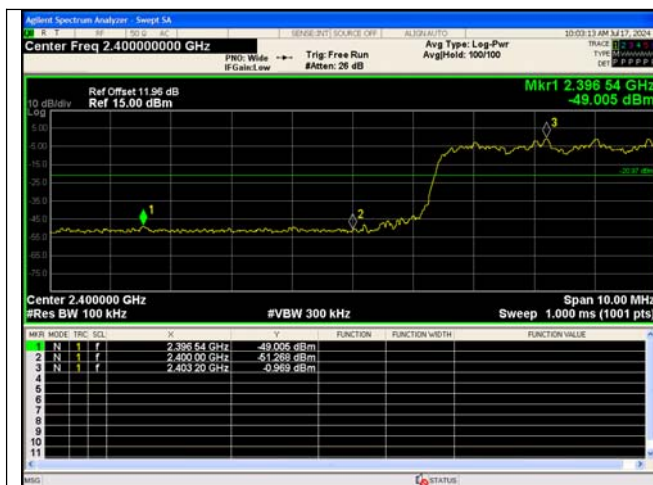
Out Of Band Emission(Left) 8DPSK_3-DH5_Channel Hopping
