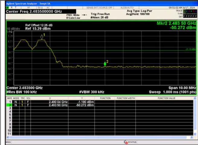
Out Of Band Emission(Right) GFSK_DH5_Channel Hopping
