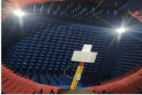
24-probe microwave anechoic chamber
