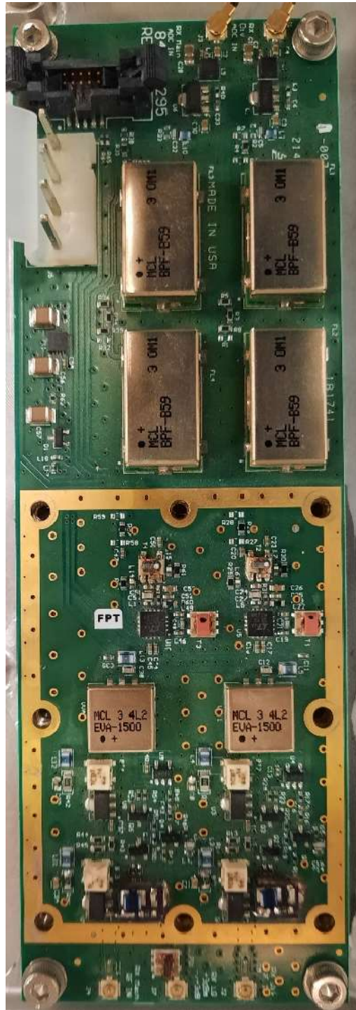
Receive Board – Top - Shield Removed
