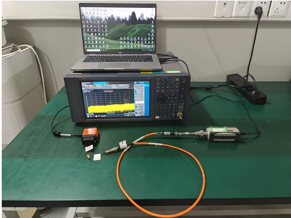
Description: Conducted Test Setup for Wi-Fi
