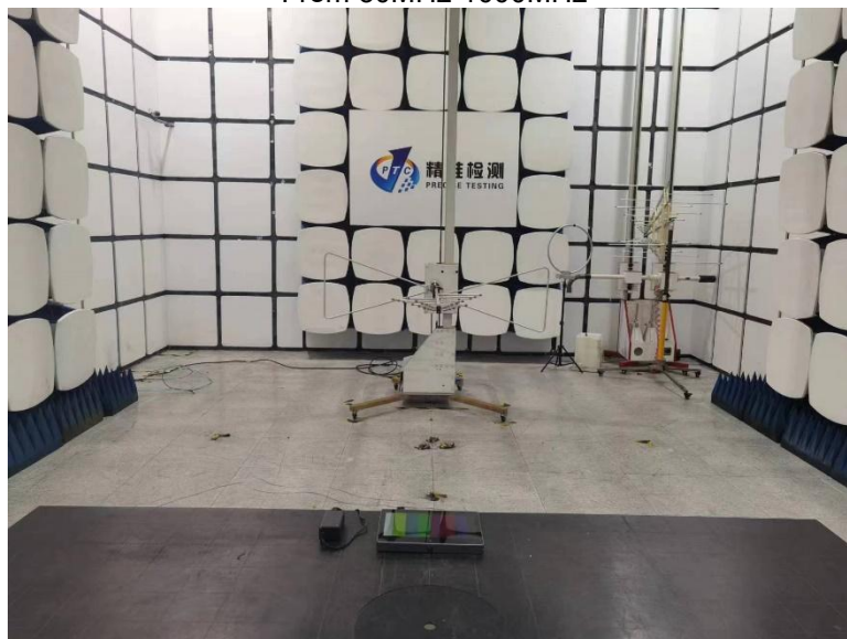
Radiated Spurious Emissions From 30MHz-1000MHz
