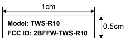
The label is displayed on the EUT by laser engraving.
