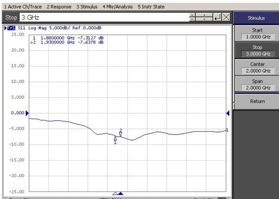
SKH8006HS(The horn is grounded without a conductive cloth 喇叭不加导电布接地)
