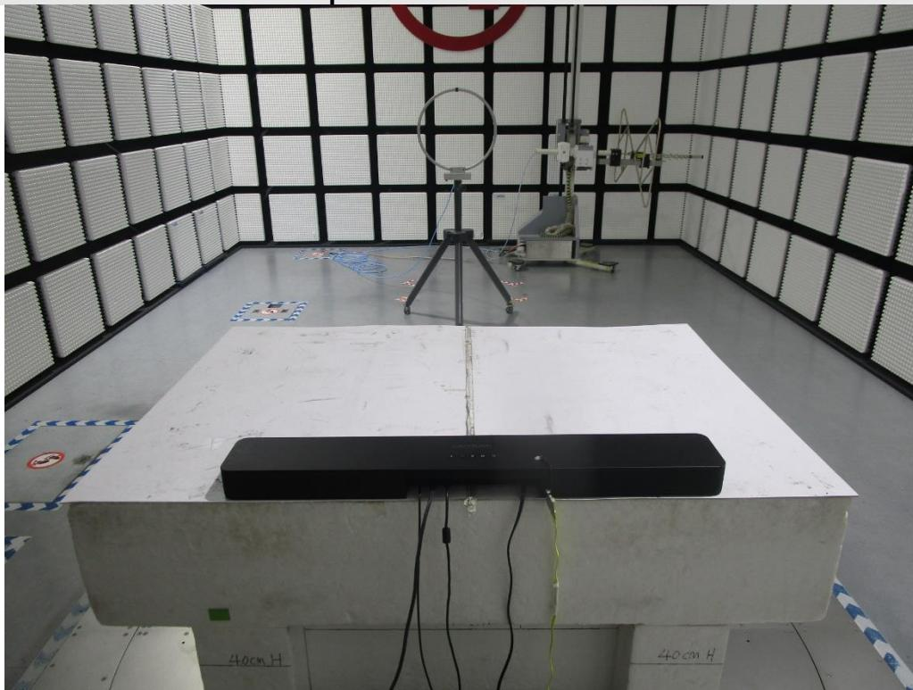
**Radiated Spurious Emission Below 1GHz and Above 30 MHz**
