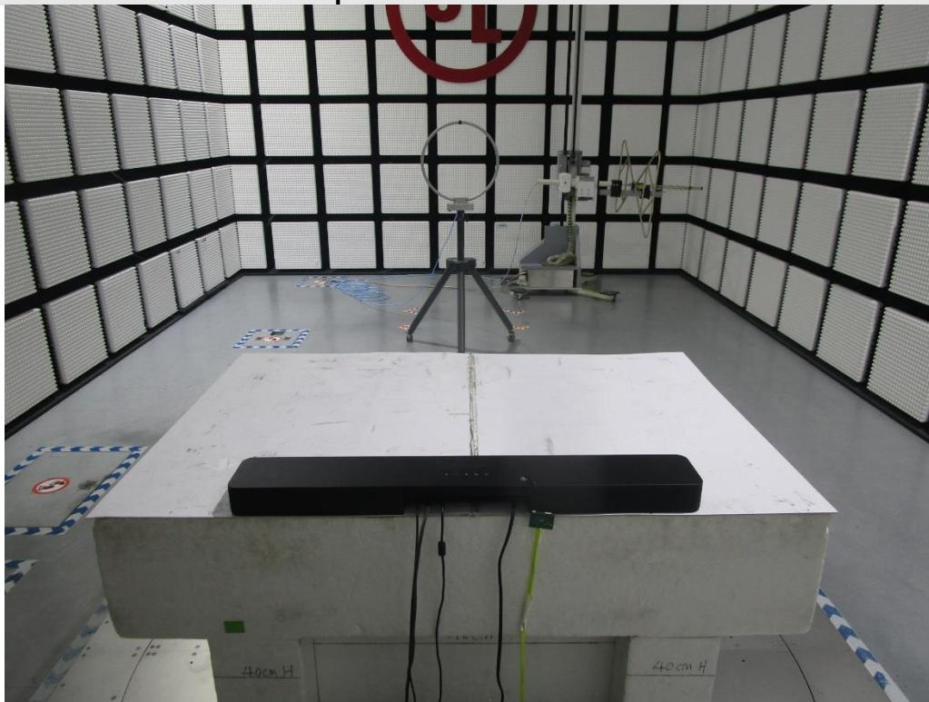
**Radiated Spurious Emission Below 1GHz and Above 30 MHz**
