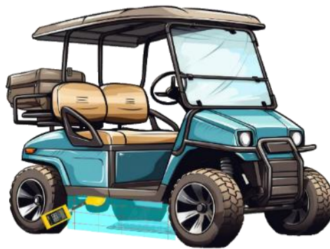
Figure 9: On-vehicle test with grid and plexiglass set so probe is centered at vehicle edge
