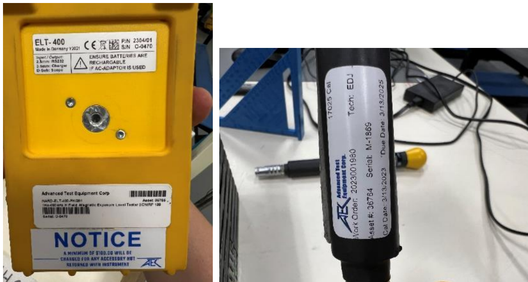
Calibrated Narda ELT-400 Meter and Probe Utilized for Testing
