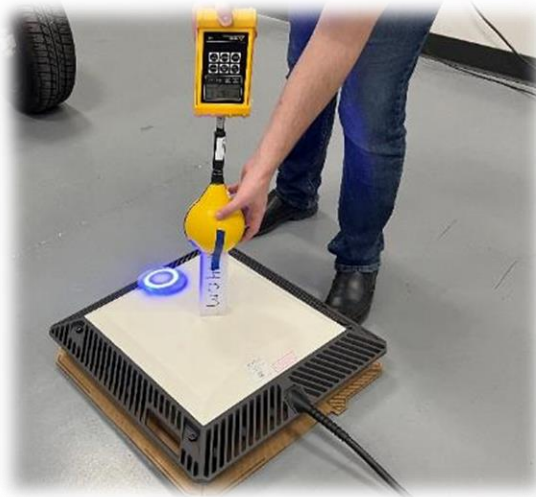
Figure 11: Field Probe Setup for Standby Measurements
