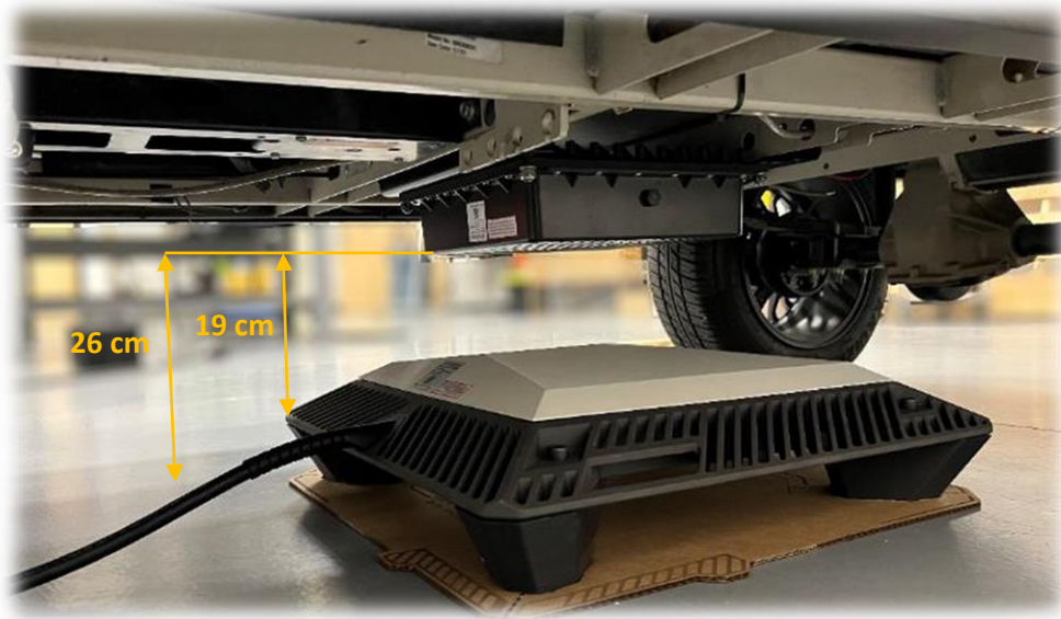
Figure 7: Receiver mounted on real vehicle with actual mounting hardware and Power Hub with 7 cm risers
