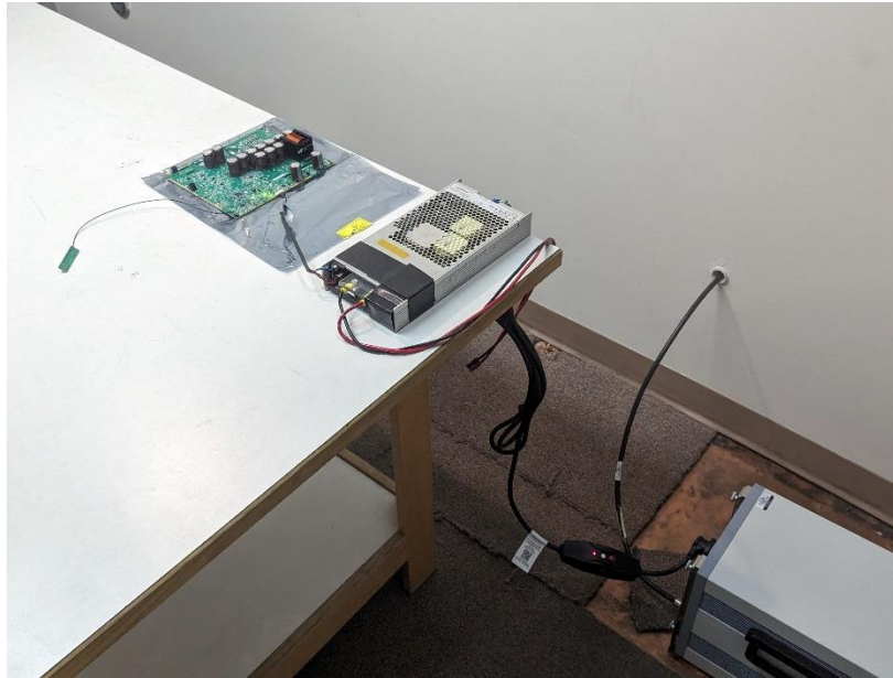
Photograph 5: Front View Conducted Emissions Worst-Case Configuration
