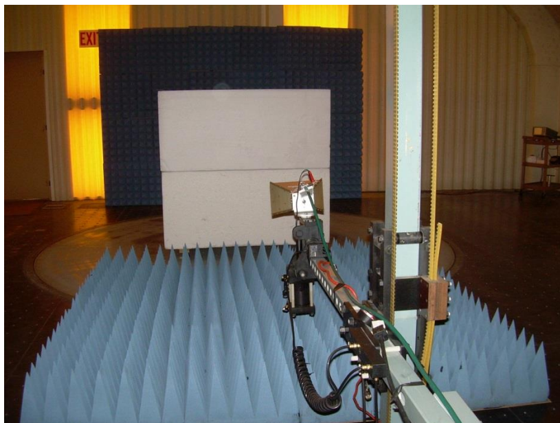
Photograph 9: Reference Photo of Test Setup for Emissions Above 1000 MHz
