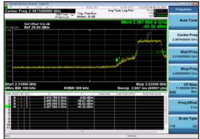
,Plot 2,Band Edge-802.11g,2462MHz ,Ant0
