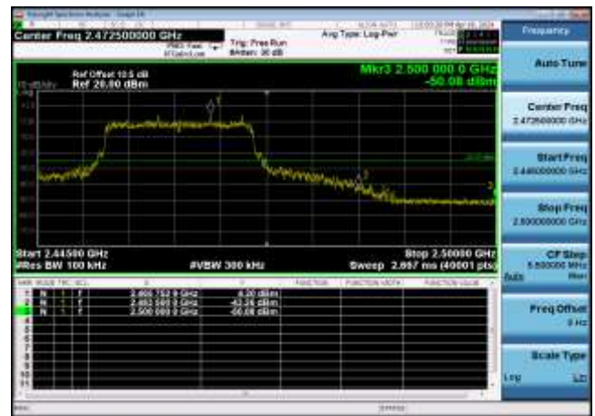
,Plot 2,Band Edge-802.11g,2462MHz ,Ant0
