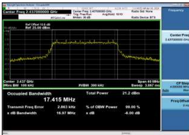
6dB Bandwidth-802.11g,2437MHz,Ant0
