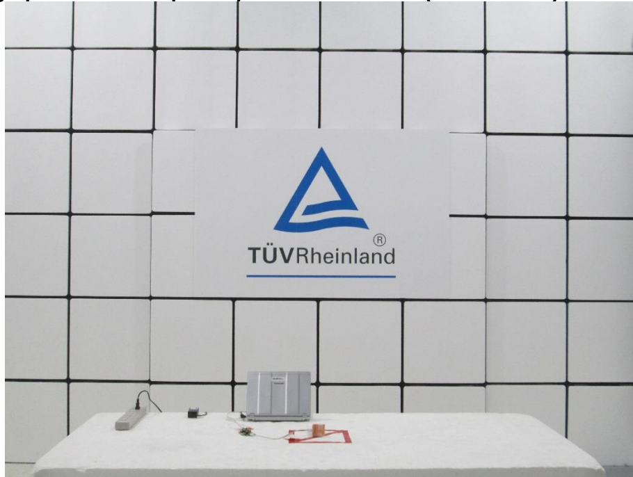
Photograph 2: Test Setup for Spurious Emissions (Front View 2)
