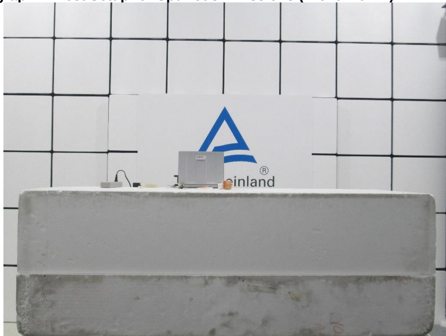
Photograph 2: Test Setup for Spurious Emissions (Front View 2)
