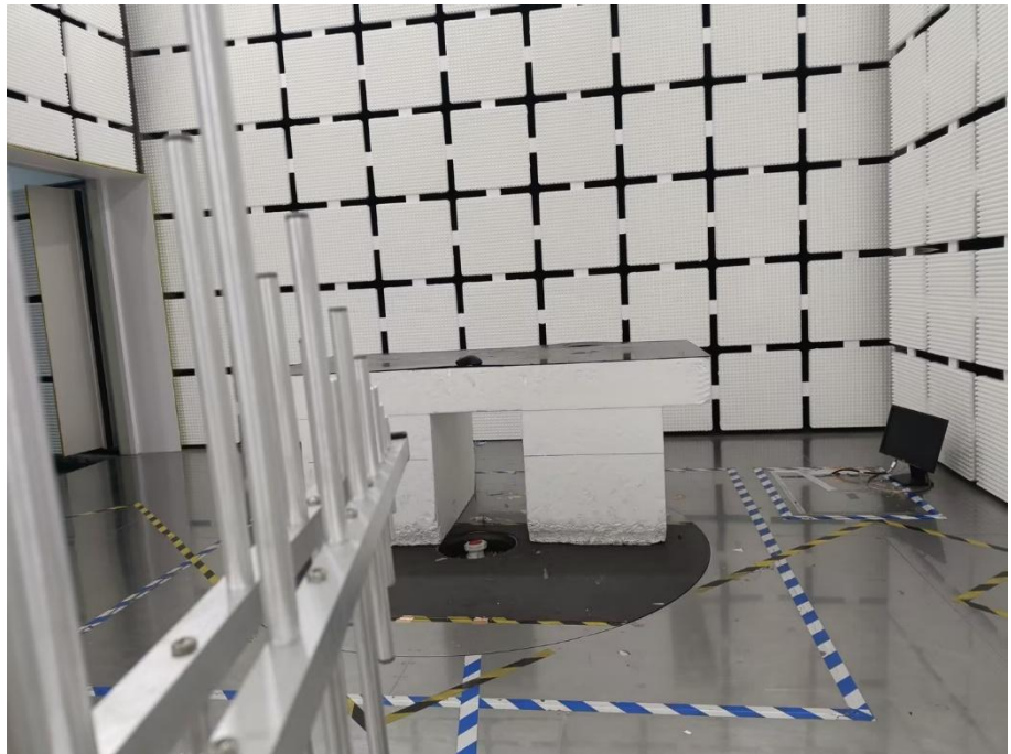
Radiation Emission Test Setup (30MHz to 1GHz)
