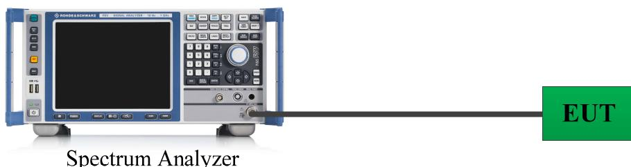
A short RF cable with low cable loss connected to the EUT antenna port, which was provided by manufacturer.
