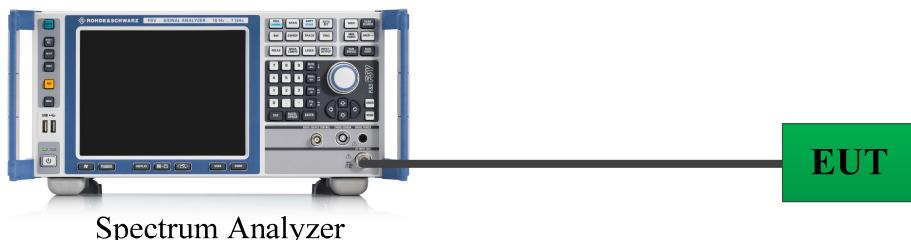
A short RF cable with low cable loss connected to the EUT antenna port, which was provided by manufacturer.
