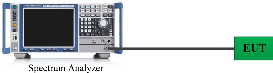
A short RF cable with low cable loss connected to the EUT antenna port, which was provided by manufacturer. The cable loss of this RF cable was offset into the setting of test equipment, which was provided by manufacturer▲.
