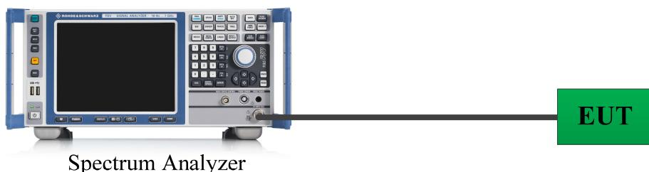
A short RF cable with low cable loss connected to the EUT antenna port, which was provided by manufacturer. The cable loss of this RF cable was offset into the setting of test equipment, which was provided by manufacturer ▲.
