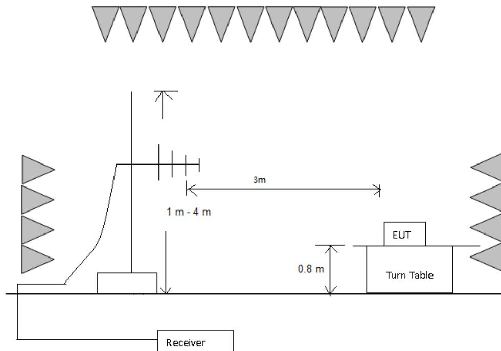
**5.2.2 Test Setup and Procedure**
