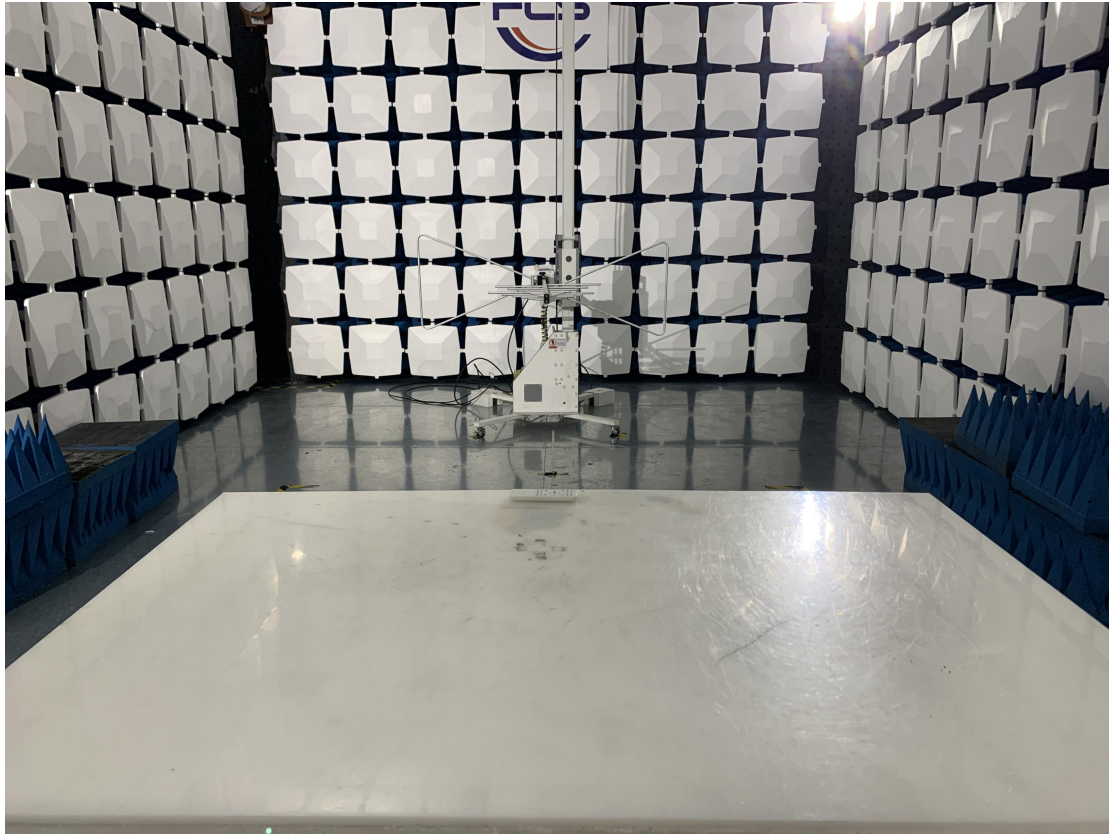
Below 1GHz for radiated emission test setup
