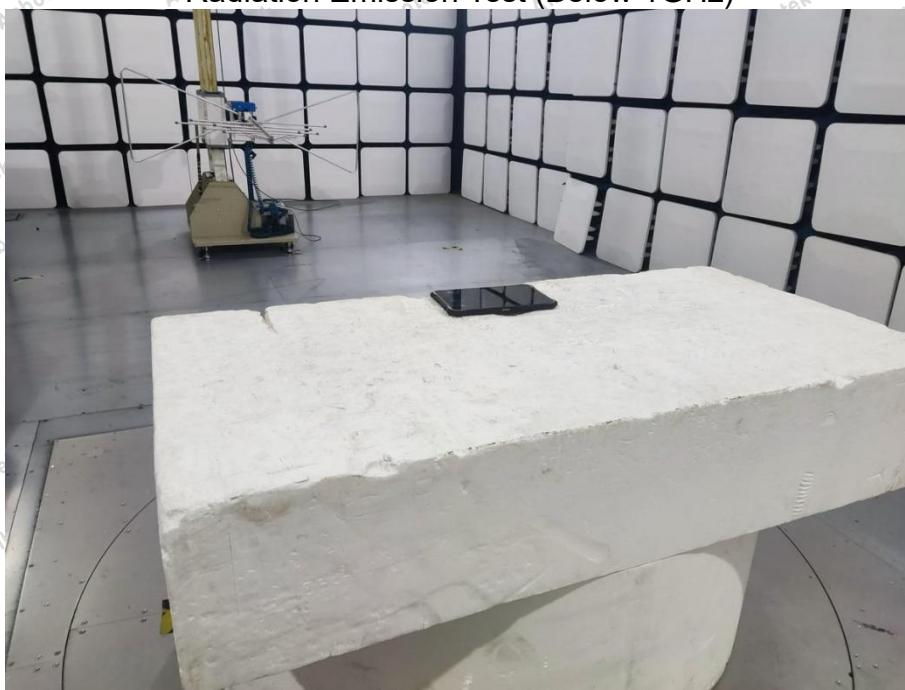
**Radiation Emission Test (Above 1GHz)**
