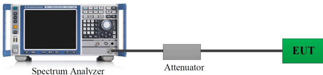
A short RF cable with low cable loss connected to the EUT antenna port, which was provided by manufacturer. The cable loss of this RF cable was offset into the setting of test equipment, which was provided by manufacturer▲.
